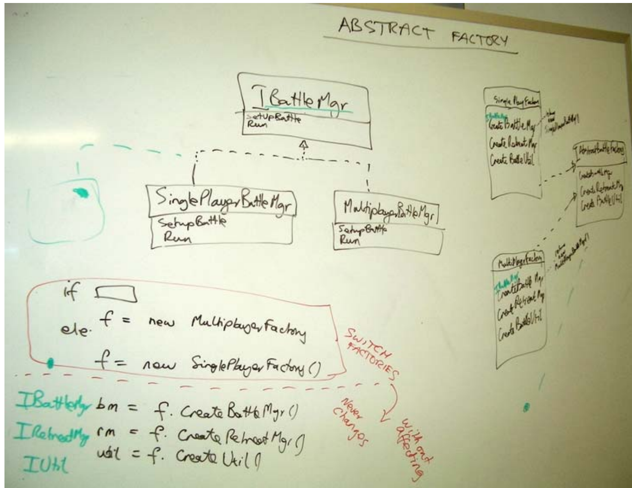
Figure 29 - Using Abstract Factory when Andy was building a computer game called "Combat Campaign". A different family of classes was required when using real battles vs. quick battles.
