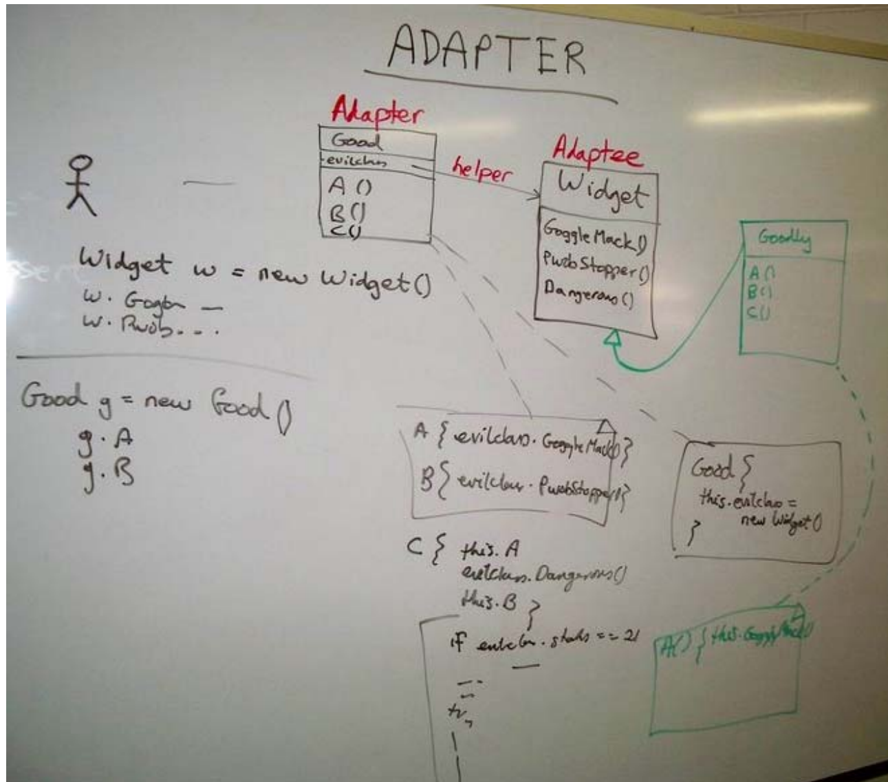
Figure 40 - Adapting the "evil class" containing bad method names like GoggleMack() and PwobStopper()
