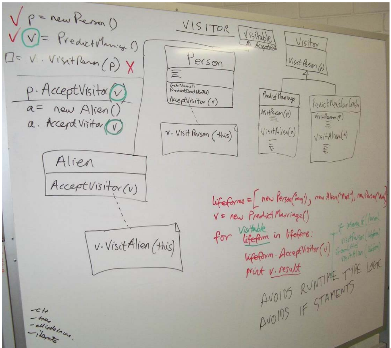
Figure 81 - Adding functionality to the Person class using Visitor Pattern
