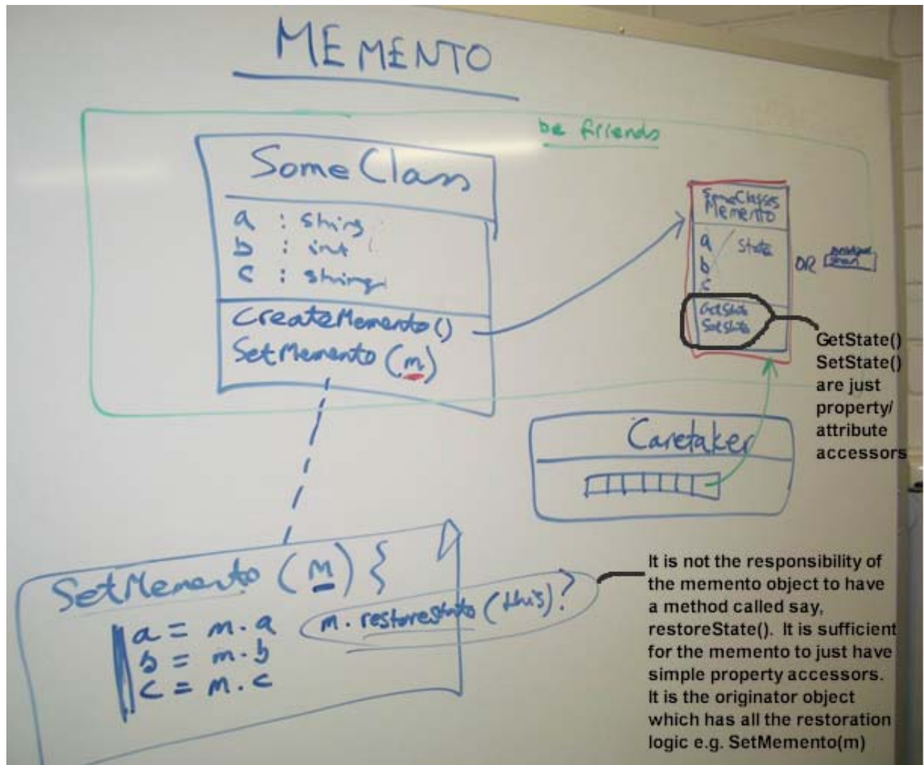
Figure 69 - Memento Idea - more detail. Note the "friends" relationship between originator and memento.
